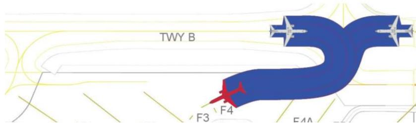
**CODE C Envergure max 36m / CODE C Max wingspan 36m**
